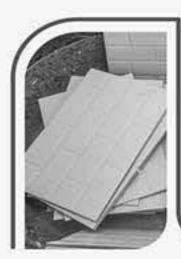
Ceramic tiles should be soaked in water, minimum 2 hrs before laying.
